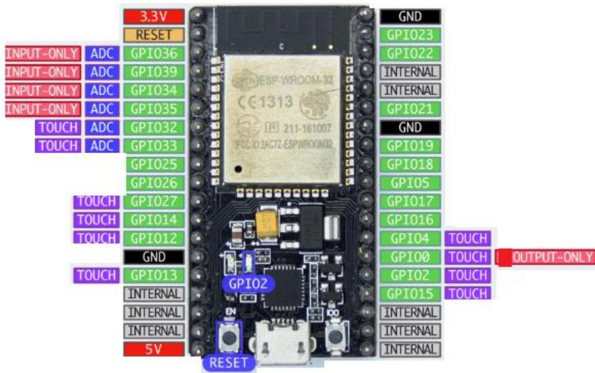
1. GPIO0 is used to determine the boot mode on startup. It should therefore not be pulled LOW on startup to avoid booting into flash mode. You can, however, still use this as an output pin.
