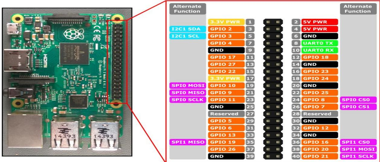
3. **GPIO Pins:** The GPIO (General Purpose Input/Output) pins are used to connect various sensors and modules to the Raspberry Pi. These pins can be configured as either input or output pins, depending on the needs of the project.
